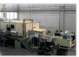
After being processed in the cold forming department the component goes to the finishing department. In this phase multi-spindle lathes and transfer machines process the item to achieve its final shape and size.
